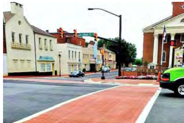
Inlaid Thermoplastic was used to create these crosswalks in Kannapolis, North Carolina. This system consists of imprinting a pattern into a heated asphalt surface. Image courtesy PatternPaving.com.
