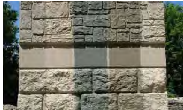
This test panel shows how various color stains can change the appearance of a noise wall. A larger precast stone pattern is used along the bottom of the test panel, with a finer texture stone pattern on top. Image courtesy FHWA.
